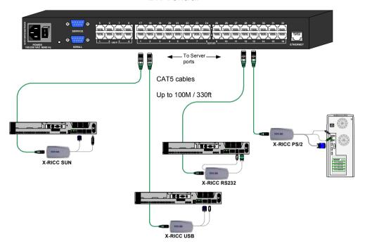
Figure 10 DX system connections
